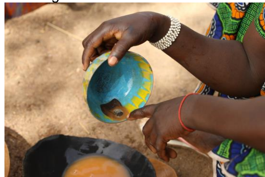
A woman drains water from a gold-mercury amalgam in Bambaraya, Senegal; April 2010. Photo: Rebecca Blackwell.
